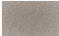
Weathered Galvalume SR=.34 E=.82 SRI=34
